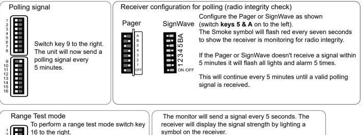
On the receiver, switch keys 5, A & B on to the left.
