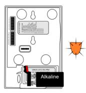
NOTE: if this is done in reverse order a low battery signal will be sent out and the test/send button will shine orange instead of green for up to 9 hours. Switch the mains off, remove the battery and reset the unit using the procedure in step 1.
